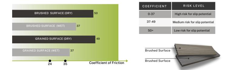
To maintain traction levels similar to the results shown, it is imperative that the deck is designed to allow proper drainage and the deck surface is kept as clean as possible.
